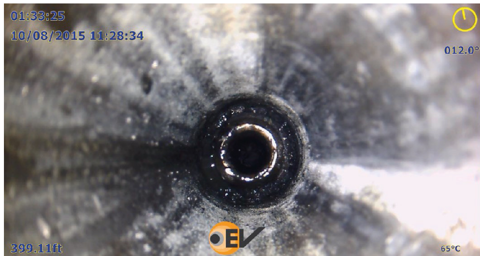
Figure 2: Top of W Slip Lock at 400 ft
