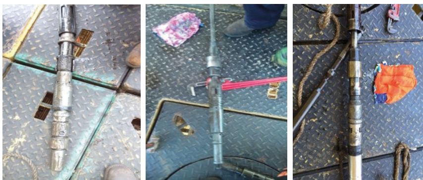
Figure 1: Fish left in hole: W Slip Lock (left), Bulldog Spear (centre), B7 (right)
